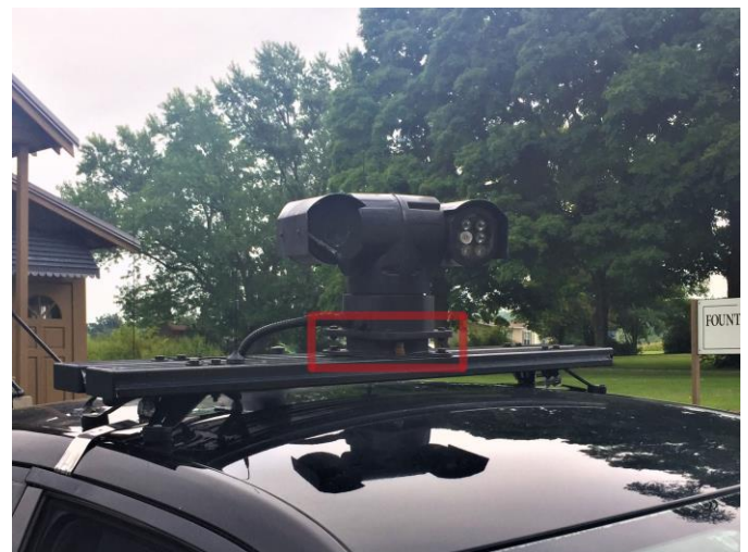
Fig. 2. The rubber cushion as showing in red.
