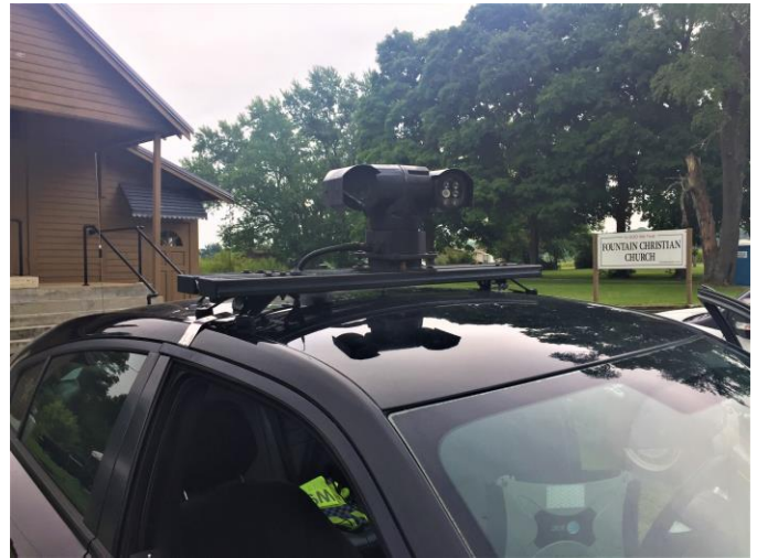
Fig. 1. The PTZ camera that been tested in this project, the lens is on the left side of the picture and the infrared unit on the right side.
